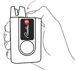
To turn Roadie on, simply press the power button at the top. To turn it off, long-press the power button for 3 seconds.
